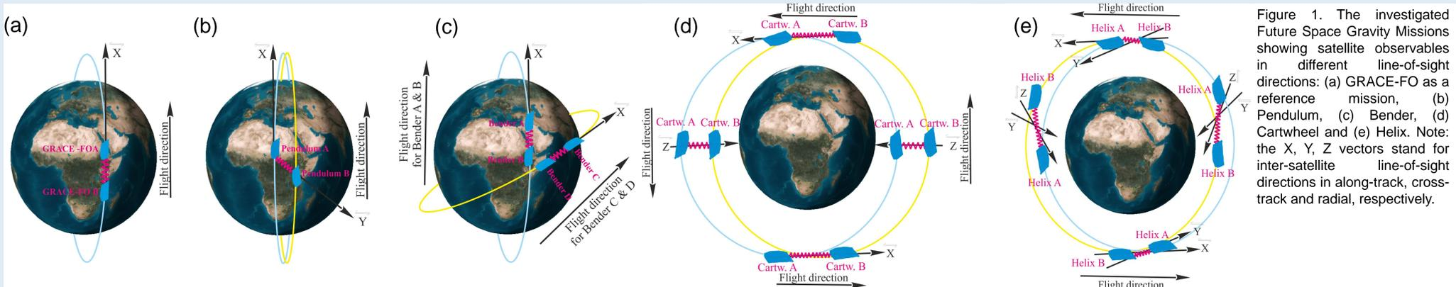
Figure 1. The investigated Future Space Gravity Missions showing satellite observables in different line-of-sight directions: (a) GRACE-FO as a reference mission, (b) Pendulum, (c) Bender, (d) Cartwheel and (e) Helix. Note: the X, Y, Z vectors stand for inter-satellite line-of-sight directions in along-track, cross-track and radial, respectively.
